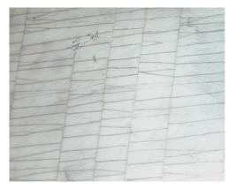
A common test method to see if your tank has undergone Ultra-violet attack is to use water based stain or marker and color in a small area that has been exposed to sunlight. This will fill any voids in the polyethylene material making cracks visible. Areas to check are the dome and lower sidewall of the tank.
