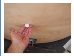
Tanks with damage similar to the picture shown below should be reported to the manufacturer, and evaluation should take place prior to the tank being placed in service.
