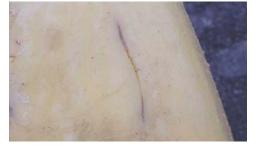
This picture is a chemical stress crack in a Crosslink polyethylene tank. Stress cracks normally develop at or near tank sidewall connections. A Crosslink tank will typically develop a stress crack prior to complete tank failure. This gives the end user warning to get the tank removed from service. Normally a Linear polyethylene tank will not give this type of warning before complete failure.
